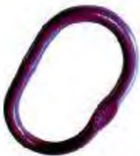
G-80 WELDED MASTER LINK ASSEMBLY A-347 Forged Alloy Steel Quenched & Tempered 1/2" -1 1/4"
