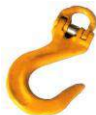
G-80 EYE SLING HOOK Forged Alloy Steel Quenched & Tempered 7mm-16mm
