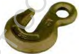
U.S. TYPE EYE GRAB HOOK Forged Carbon or Alloy Steel Quenched & Tempered 1/4" -3/4"
