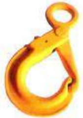
G-80 NEW CLEVIS SELF-LOCKING SAFETY HOOK Forged Alloy Steel Quenched & Tempered 7/8mm-16mm
